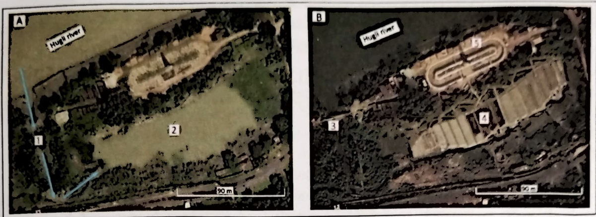
Figure 1: Components of the brick kiln at Akra in (A) Monsoon season (B) Pre-monsoon season 1. Water inlet 2. Sediment reservoir 3. Reconstructed embankment 4. Drying area 5. Furnace. Blue line in (A) indicates the passage of river water through inlet towards reservoir
